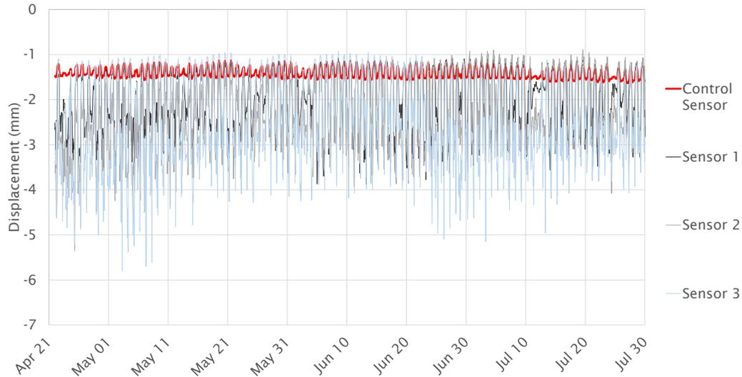
*Displacement readings of sensors installed in Brand B polyiso in 2015. Note that the red line, Control Sensor, represents the readings from the sensor that was installed with its plunger in a fixed position.*
