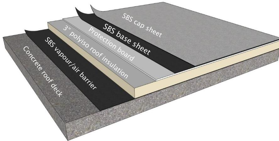
*Figure 3.2 Schematic of the conventional roof assembly installed at the study building.*
