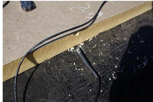
*Figure 3.9 Closeup of RH and temperature sensor that was installed into top surface of polyiso insulation.*
