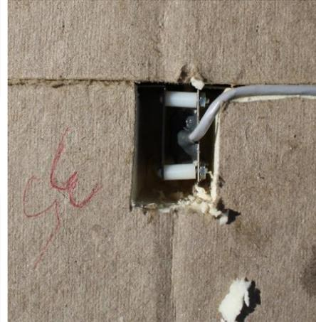
*Figure 3.7 Displacement sensor installed at joint between adjacent polyiso insulation boards. The plunger is now depressed and in contact with the plate on the adjacent board.*
