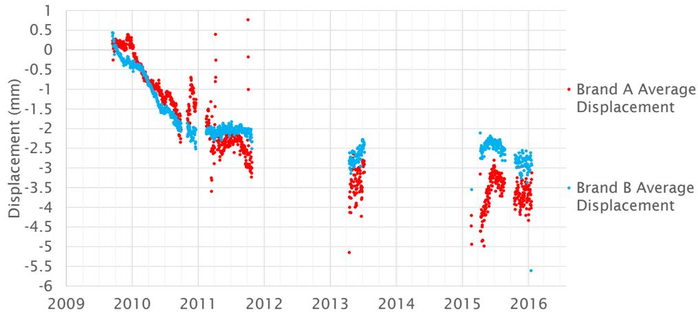
Figure 3.16 Dimensional change of Brand A and Brand B polyiso throughout the monitoring period.
