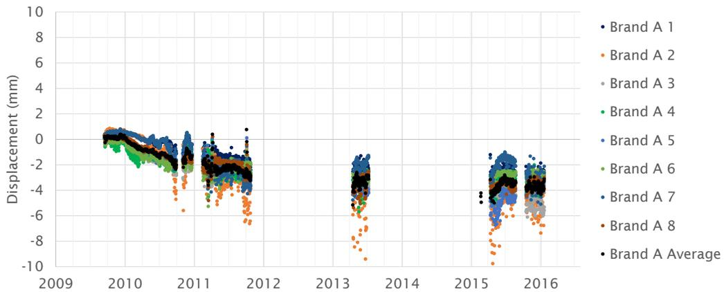
Figure 3.12 Brand A polyiso dimensional change over time for the 8 monitored locations. Note that the monitoring system was turned off during the time periods with no data.
