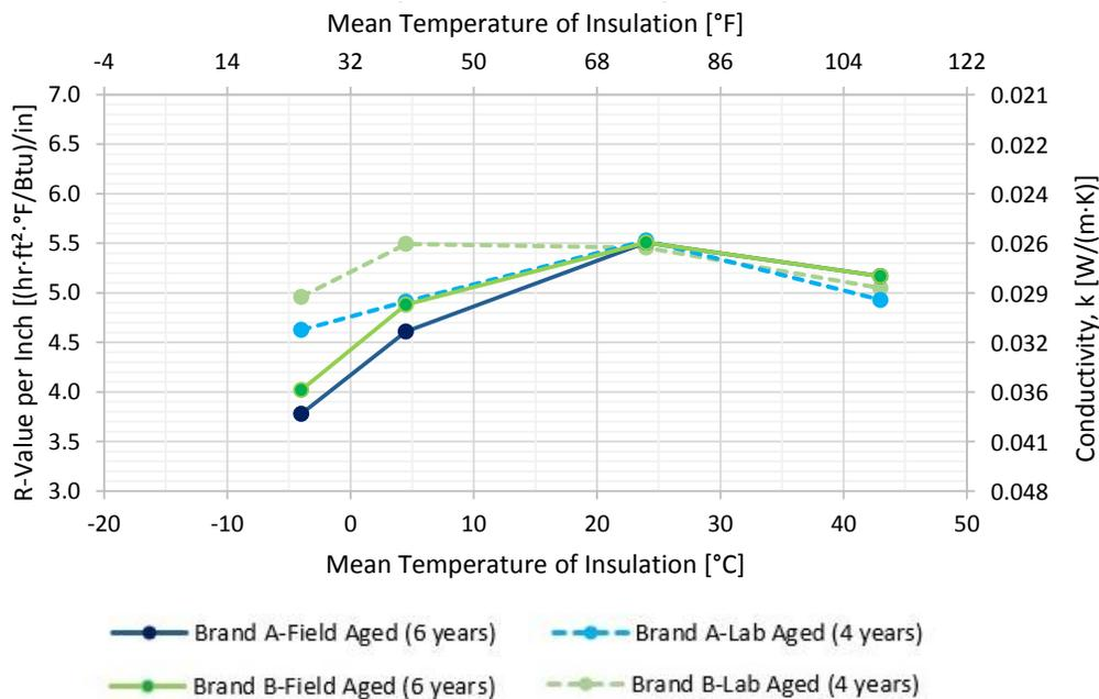
Figure 4.1 Chart of measured polyiso insulation thermal performance at various different temperatures
