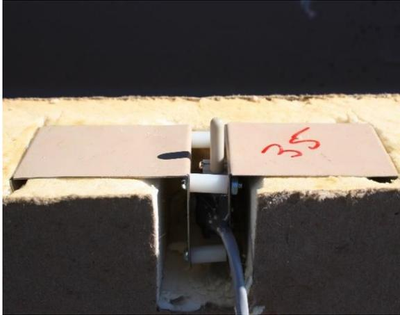
*Figure 3.6 Displacement sensor Installed into the edge of a polyiso insulation board with the plunger fully extended. The plunger will contact the contact plate on the adjacent insulation board once installed.*
