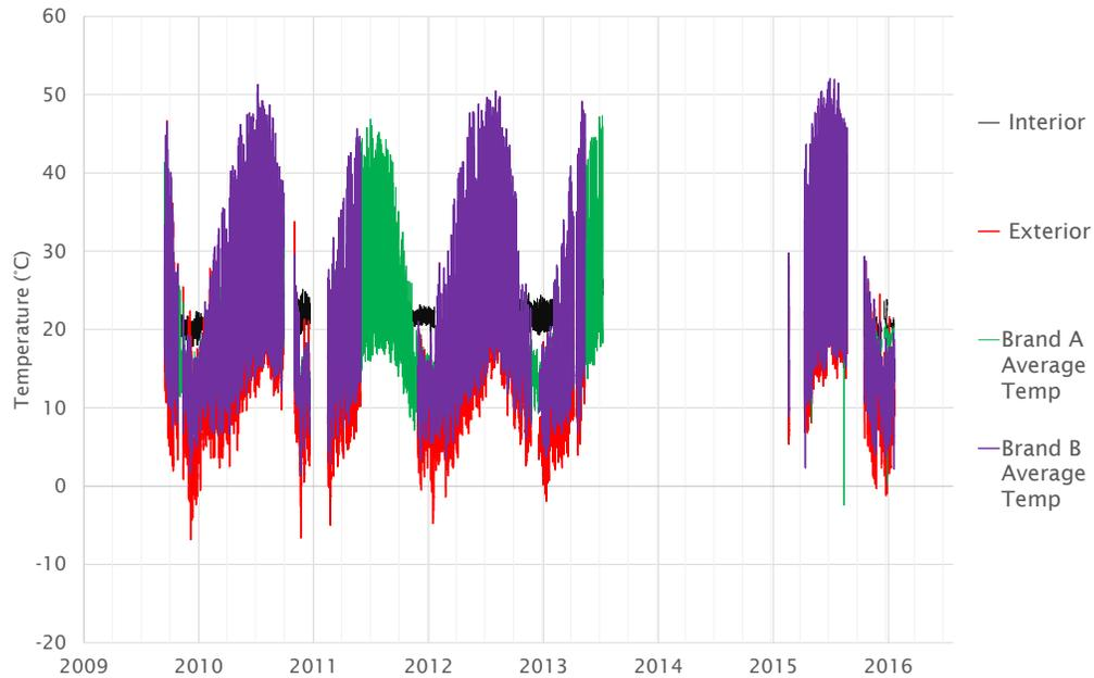
Figure 3.17 Temperature average of Brand A and Brand B polyiso, compared to interior and exterior temperature during the monitoring period.
