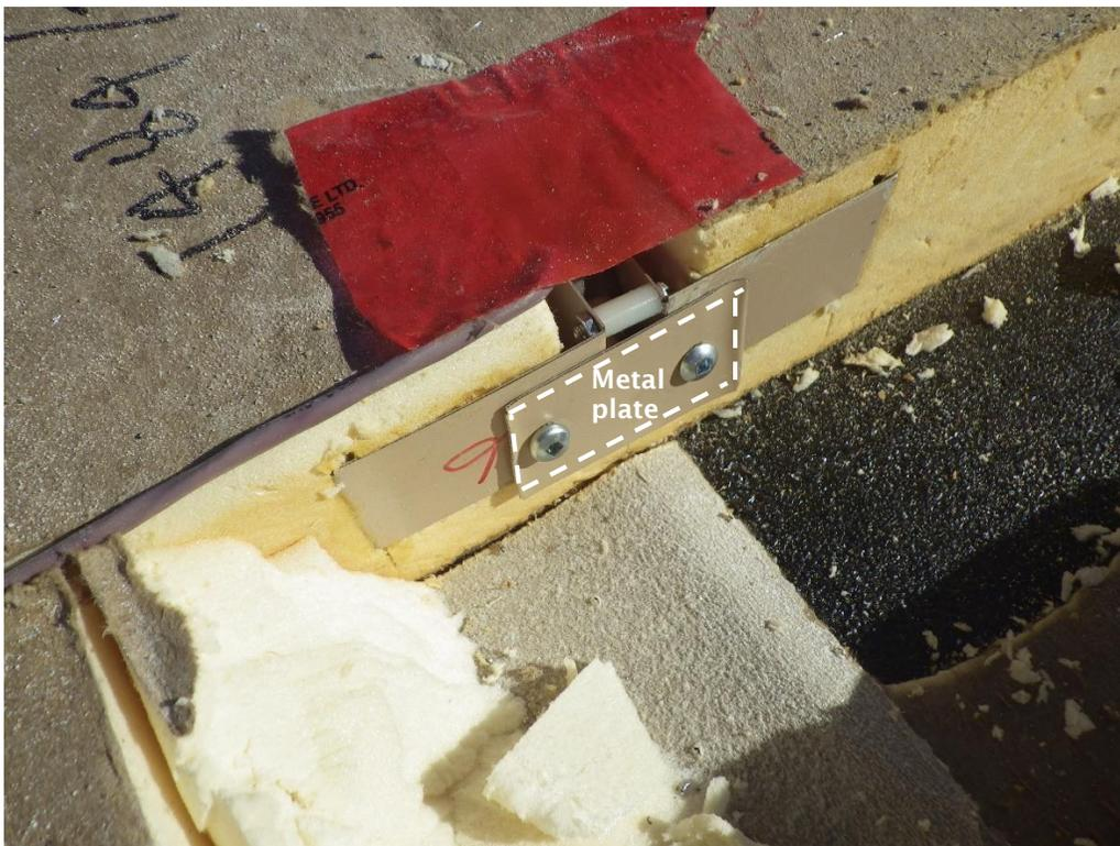
*Displacement sensor with plunger restrained by rigid metal plate at consistent position in order to determine the temperature sensitivity of its readings.*
