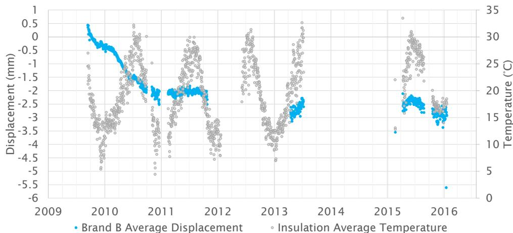
Figure 3.15 Brand B polyiso roof insulation average displacement throughout the 6-year monitoring period, plotted alongside the average temperature recorded at the core of the insulation.
