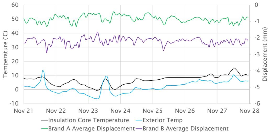
Figure 3.19 Dimensional movement of polyiso during representative week of cold weather from November 21<sup>st</sup> to 28<sup>th</sup> 2010.
