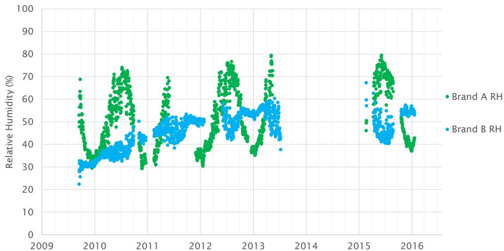
Figure 3.20 Relative humidity of Brand A and Brand B during the monitoring period.
