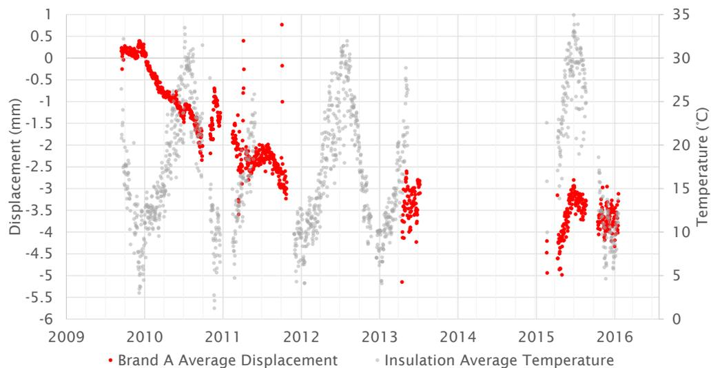
Figure 3.13 Brand A polyiso roof insulation average displacement (dimensional change) throughout the 6-year monitoring period, plotted alongside the average temperature recorded at the core of the insulation.
