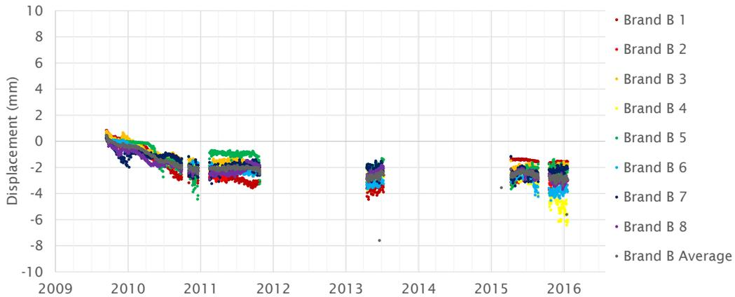
Figure 3.14 Brand B polyiso dimensional change over time for 8 monitored locations. Note that the monitoring system was turned off during the time periods where no data is shown.
