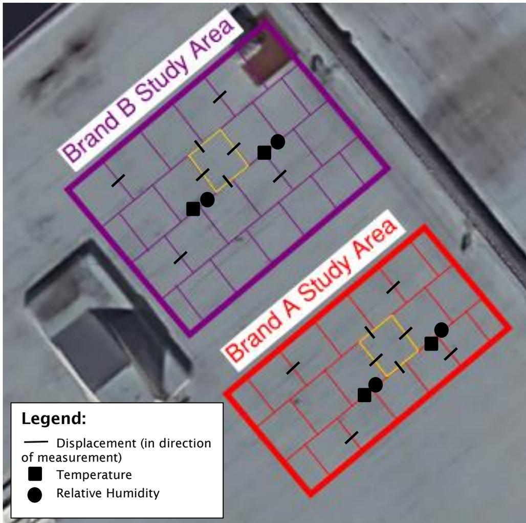
Figure 3.4 Location of sensors installed in roof assembly at test building in New Westminster, BC.
