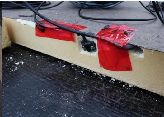
*RH, temperature and moisture sensors installed into polyiso insulation.*
