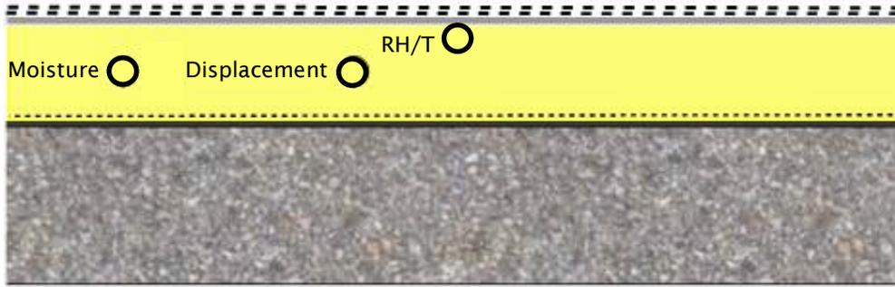
Figure 3.5 Schematic of sensor installation location within the roof assembly. Note that moisture and displacement sensors were installed at the core of the 3" polyiso roof insulation boards whereas the RH/T sensors were installed at the top.
