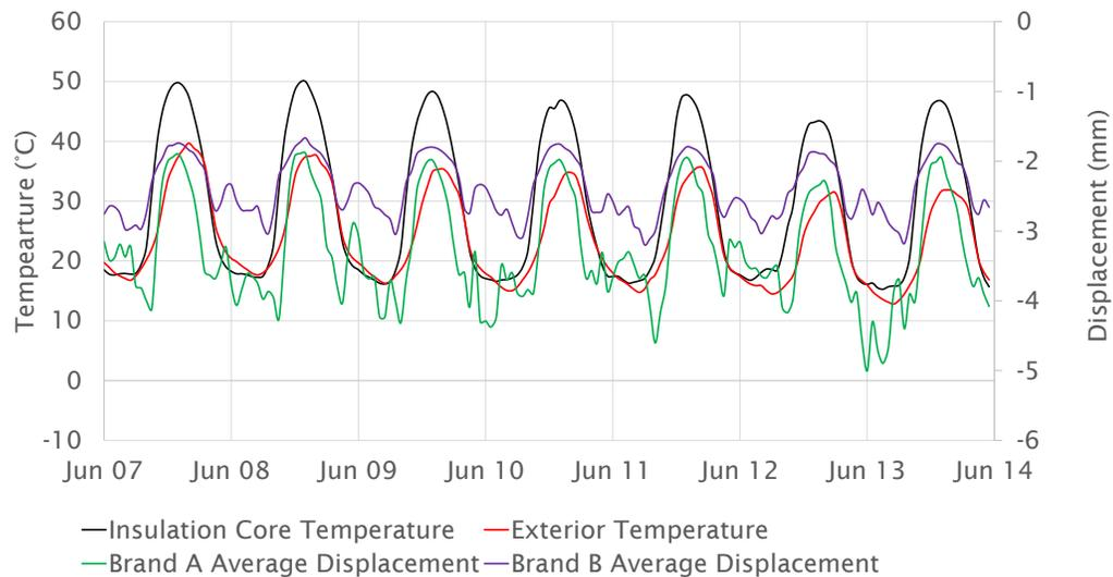
Figure 3.18 Dimensional movement of polyiso during representative week of hot weather from July 7<sup>th</sup> to 14<sup>th</sup>, 2015.
