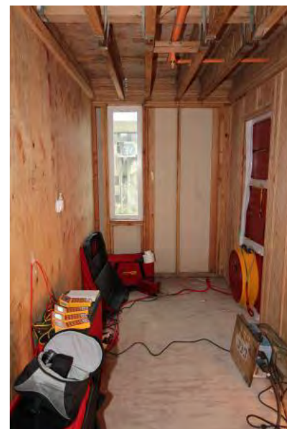
Air-leakage testing of a single suite in a wood-frame MURB. Testing is often performed as part of building commissioning to measure the enclosure airtightness as well as the compartmentalization of the individual suites prior to whole building airtightness testing.
