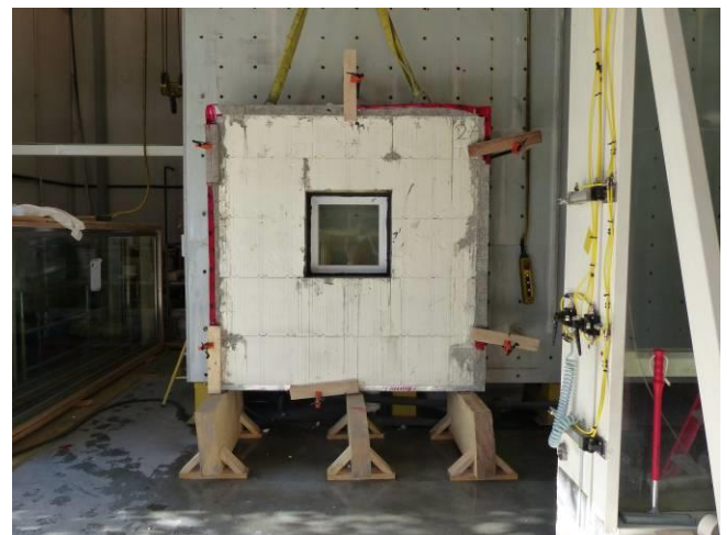
Fig. 4.3.1 Water Testing on Module 2A
