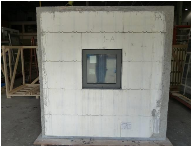
Fig. 2.2.1 Module 1A – Internal with Buck Flashing
