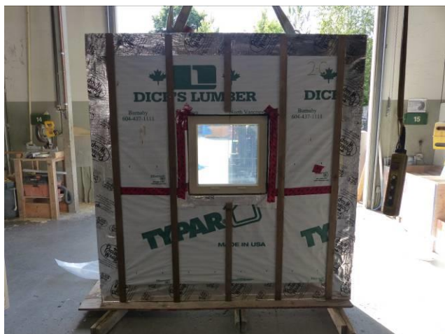
Fig. 2.2.5 Module 2C – Benchmark – Sheathing Paper with Vertical Strapping
