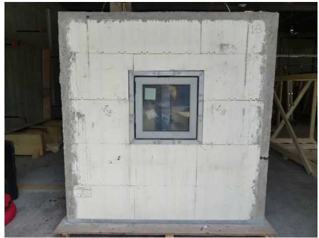
Fig. 2.2.2 Module 1B – External with Buck Flashing
