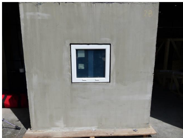
Fig. 2.2.4 Module 2B – EIFS Basecoat
