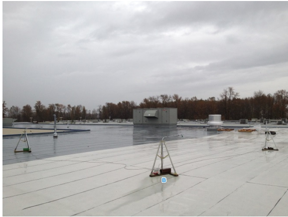
Figure 10 Reflected solar radiation sensors (3 in total) located at grey and white roof (2 locations).
