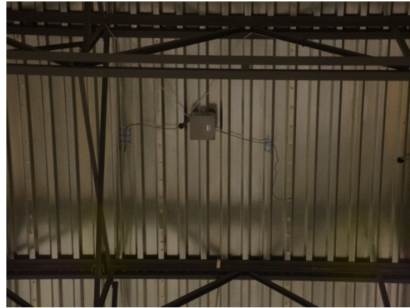
Figure 11 Interior view of data-logger and two interior temperature sensors (metal deck) and surrounding air. Deck flutes run in north-south direction.
