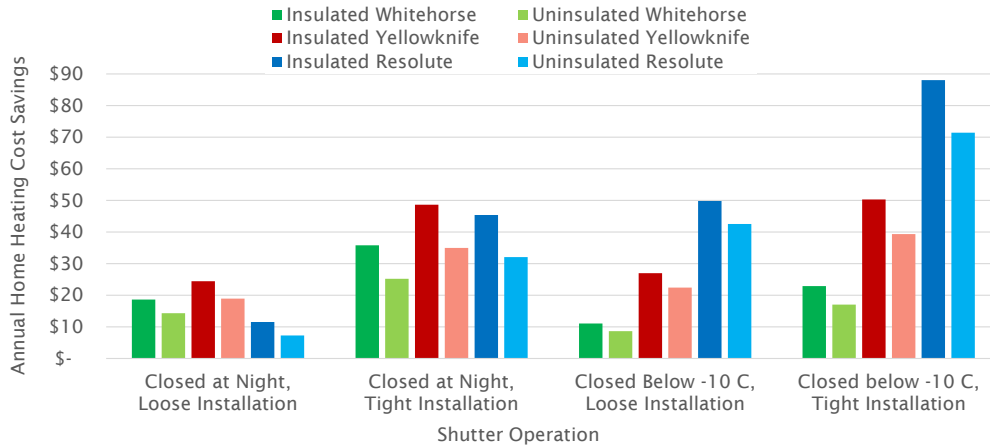
Figure 4.9 Typical heating energy savings for a house with various exterior shutter configurations compared to a house without exterior shutters. Insulated shutters (RSI-2 or R-11) versus uninsulated (RSI-0.2 or R-1) are shown. “Tight” installation refers to shutters that are installed as airtight as possible against the wall or window; “loose” installation refers to cases where outdoor air bypasses the shutters.
