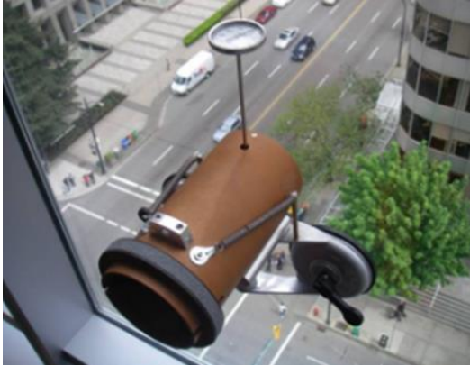
Figure 9: Performing a Frost Point test on a suspect unit.
