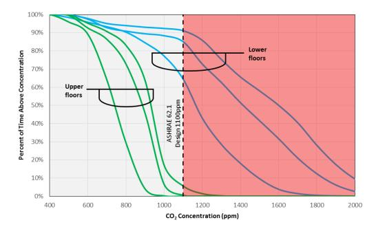
Figure 5: Fraction of time the average suite  $CO_2$  level is above a given concentration
