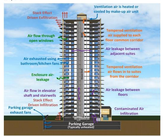
Figure 1: Overview of components of airflow and ventilation in a multi-unit residential building
