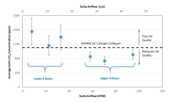
*Figure 4: Air quality differences between floors due to uneven airflow distribution*
