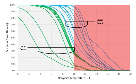
Figure 8: Percentage of time the dew point temperature is above a given threshold during the heating season in suite entrance doorways
