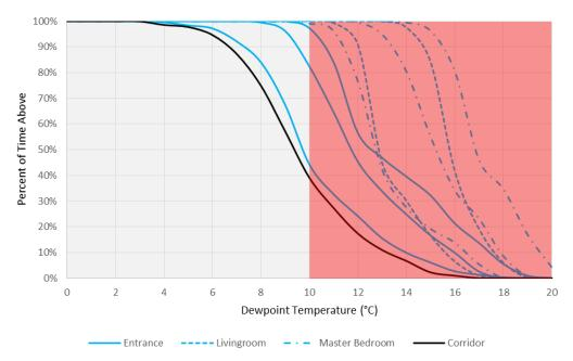
Figure 9: Percentage of time the dew point is above a given threshold during the heating season throughout suites on a lower floor
