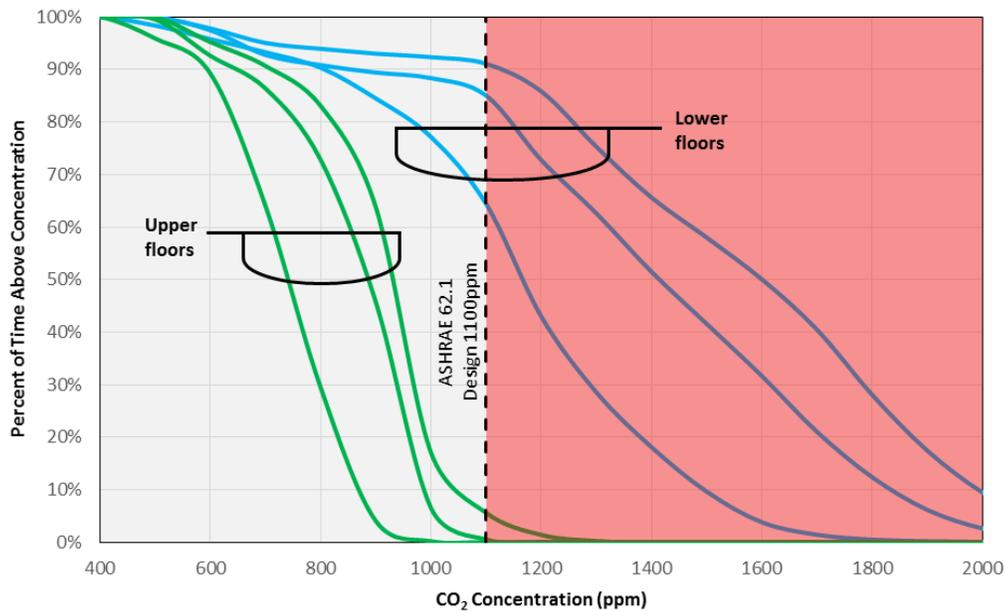
Figure 5: Fraction of time the average suite CO<sub>2</sub> level is above a given concentration
