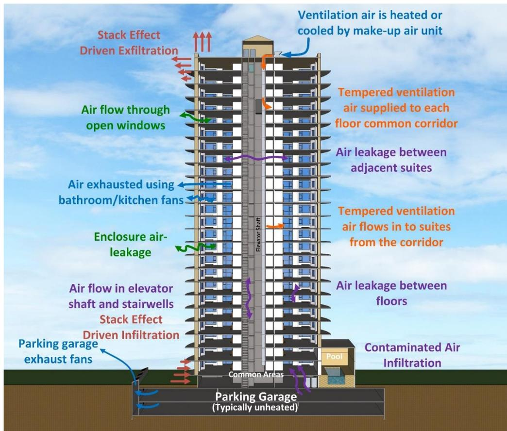
Figure 1: Overview of components of airflow and ventilation in a multi-unit residential building
