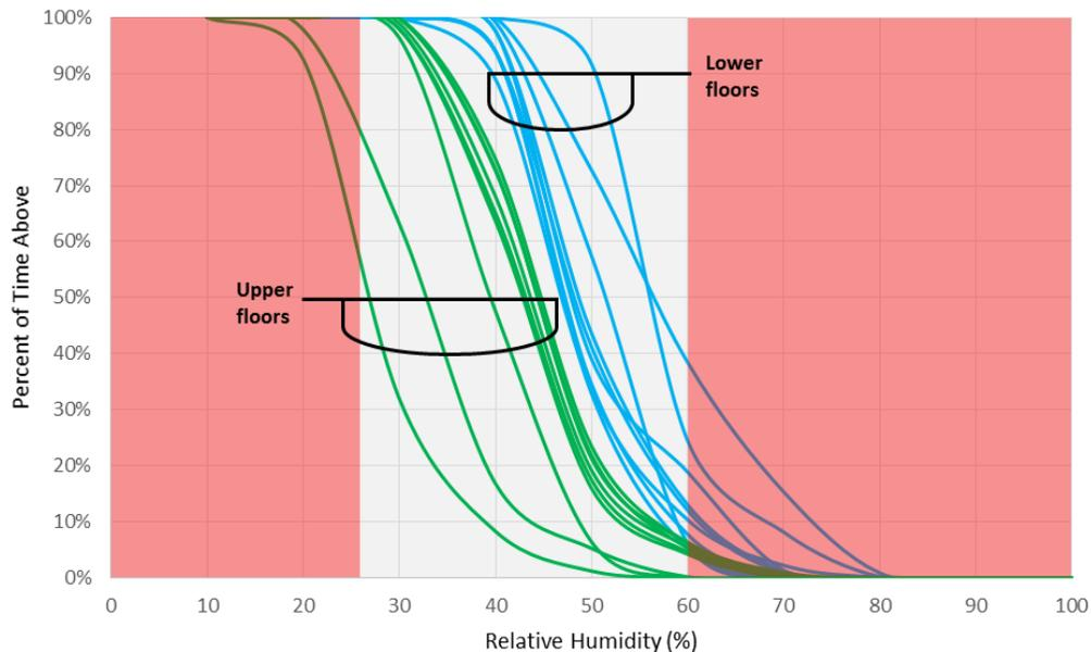
Figure 10: Percentage of time relative humidity is above an indicated threshold during the heating season
