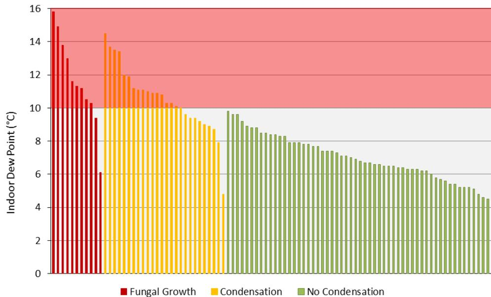
Figure 6: Indoor dew point temperature measured in suites with fungal growth, condensation, or no condensation during the heating season in Vancouver, BC
