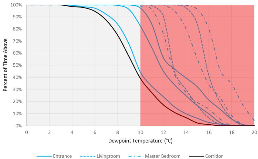
Figure 9: Percentage of time the dew point is above a given threshold during the heating season throughout suites on a lower floor
