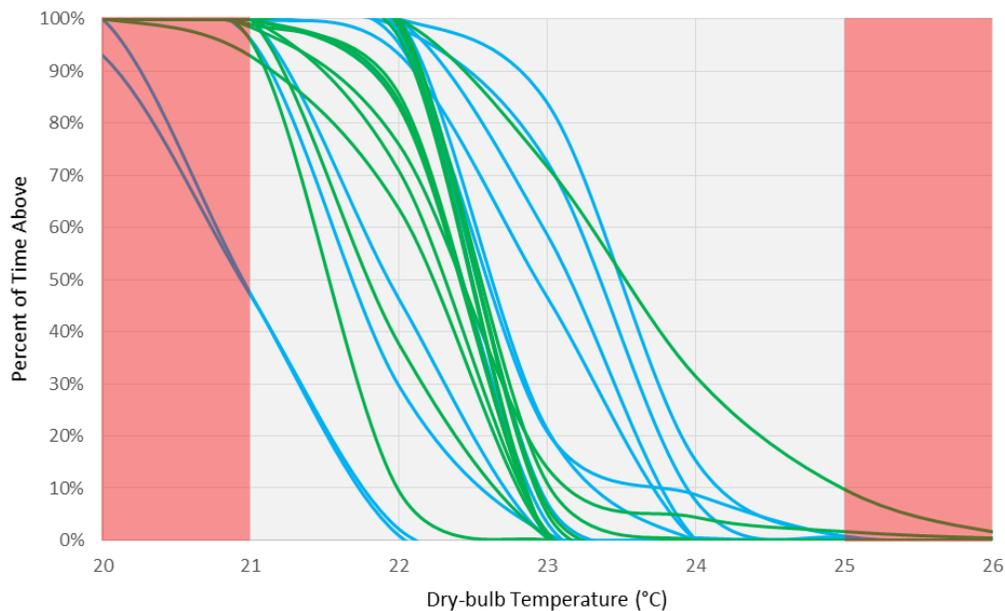
Figure 11: Percentage of time dry-bulb temperature is above an indicated threshold during the heating season. (Suites in upper floors are presented in green and lower floors in blue).
