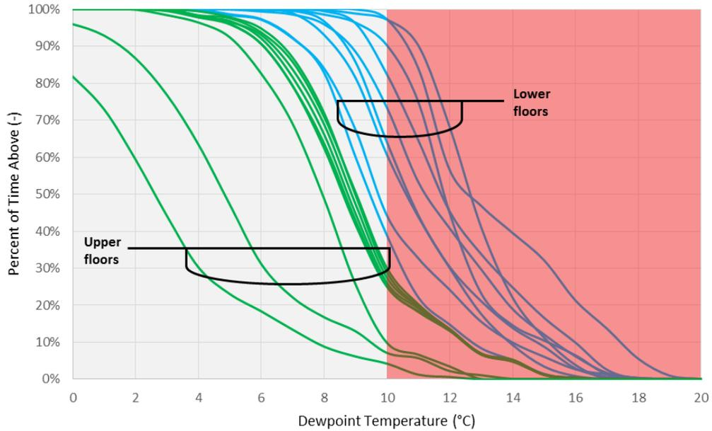
Figure 8: Percentage of time the dew point temperature is above a given threshold during the heating season in suite entrance doorways
