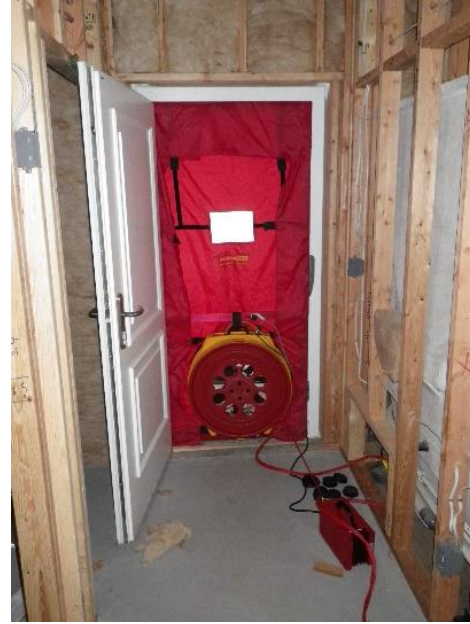
Figure 1-1 Example of fan door equipment used for airtightness testing of Part 9 housing.
