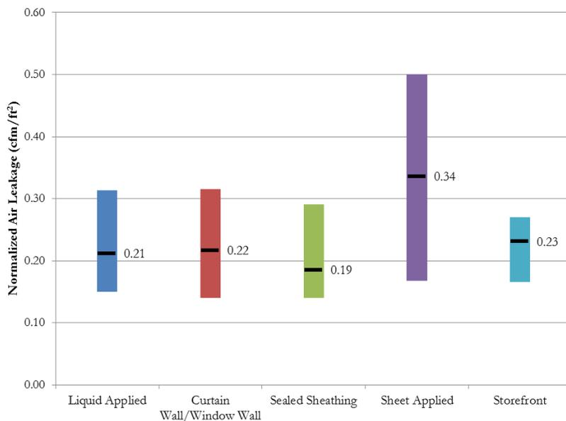
**Figure 4** Minimum, maximum, and average leakage results for each air barrier type. Average values shown as black dashes. The previously mentioned outlier has been omitted.
