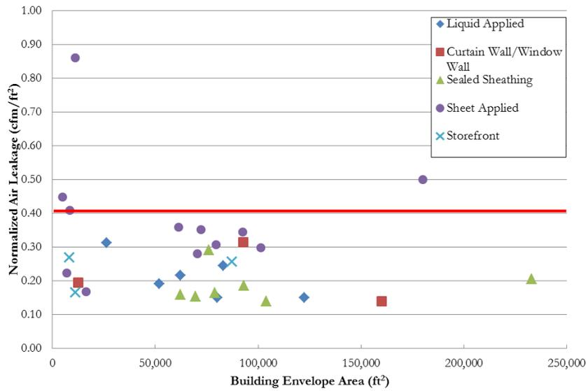
**Figure 3** Normalized Leakage Area plotted against Building Enclosure Area. Marker types denote different air barrier types.
