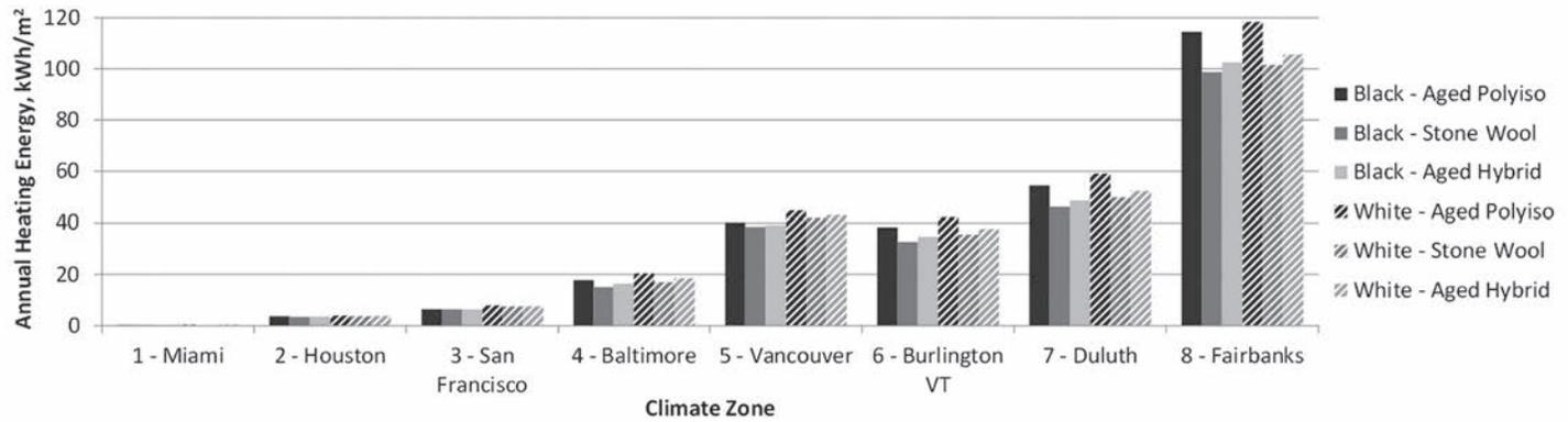
**Figure 19 – Commercial retail building annual heating energy use intensity in eight climate zones.**
