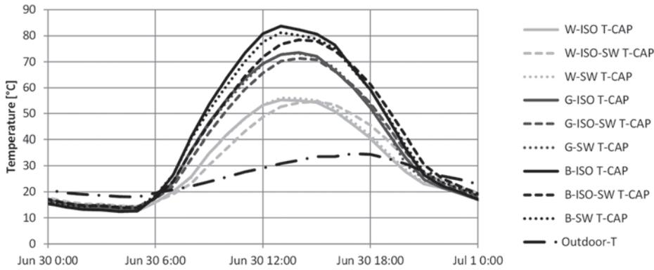
Figure 15 – Roof membrane cap sheet temperature for nine monitored roof assemblies – June 30, 2013 (summer).
