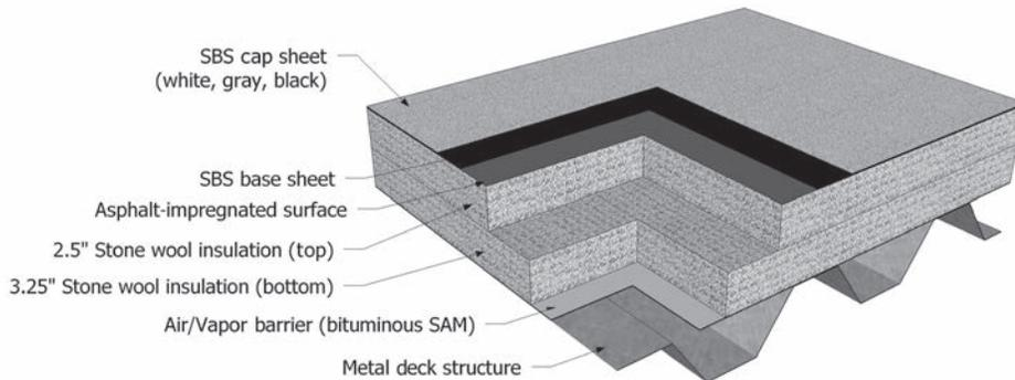
**Figure 3 – Stone wool roof assembly (5.75 in. stone wool, R-21.4); weight: 26.7 kg/m<sup>2</sup>, heat capacity: 22.7 kJ/K/m<sup>2</sup>.**
