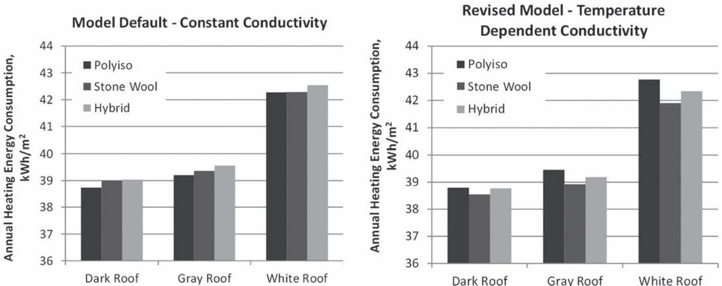
Figure 17 – Impact of modeling constant roof insulation conductivity (left) and temperature-dependent conductivity (right) for retail building in Vancouver.
