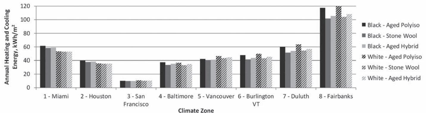
**Figure 21 – Commercial retail building annual combined heating and cooling energy use intensity in eight climate zones.**
