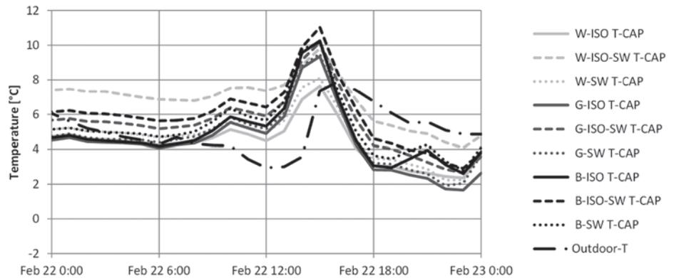
**Figure 11 – Roof membrane cap sheet temperature for nine monitored roof assemblies – Feb. 22, 2013 (winter).**
