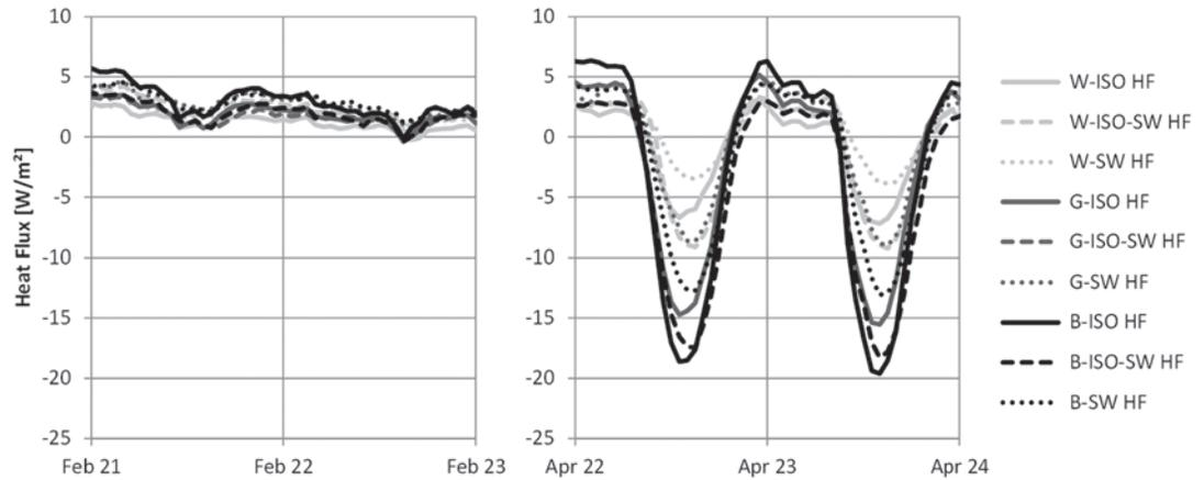
Figure 8 - Heat flux measurements through each roof assembly - February 21-23, 2013 (winter) and April 22-24, 2013 (spring cool). Note: G-ISO-SW data unavailable during April 22-24 period.
