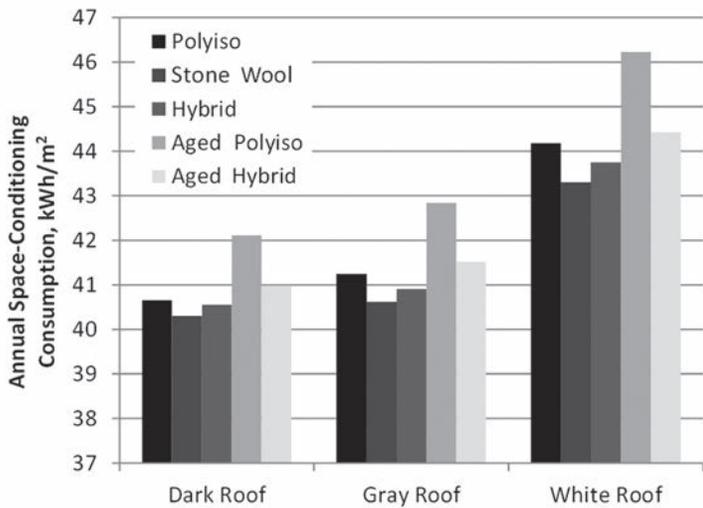
**Figure 18 – Impact of modeling aged conductivity of polyisocyanurate insulation on total building energy consumption in Vancouver.**
