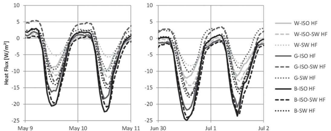
Figure 9 - Heat flux measurements through each roof assembly - May 9-11, 2013 (spring warm) and June 30 - July 2, 2013 (summer peak design). Note: Potential error offset with G-ISO-SW and G-SW heat flux data during time period.
