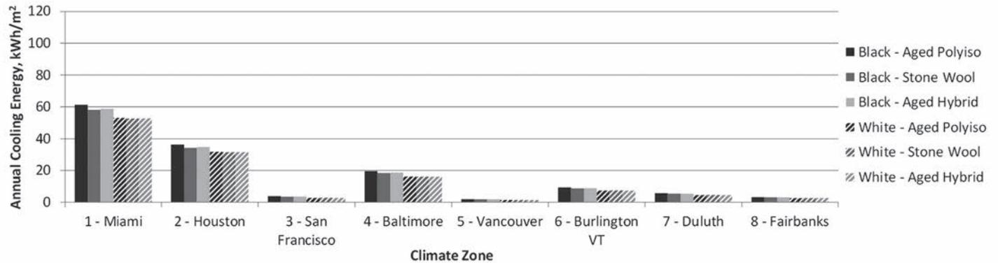
**Figure 20 – Commercial retail building annual cooling energy use intensity in eight climate zones.**
