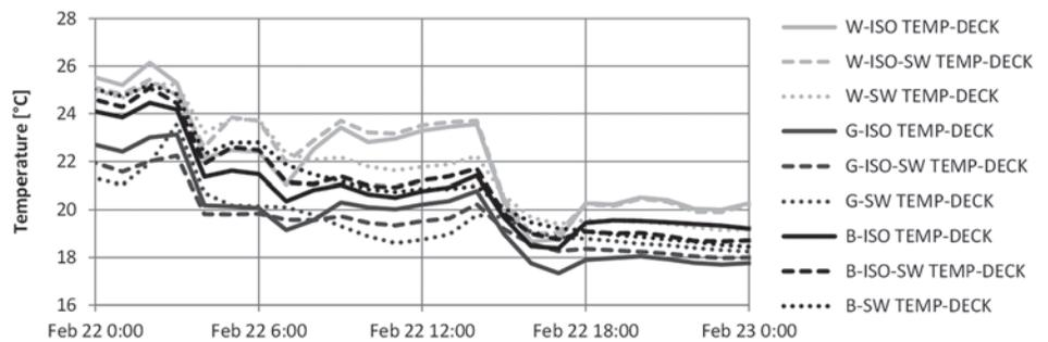
**Figure 12 – Interior metal roof deck surface temperature for nine monitored roof assemblies – Feb. 22, 2013 (winter).**
