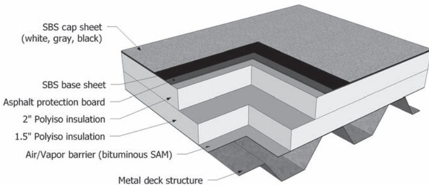
**Figure 2 – Polyisocyanurate roof assembly (3.5 in., R-21.5); weight: 4.6 kg/m<sup>2</sup>, heat capacity: 6.75 kJ/K/m<sup>2</sup>.**
