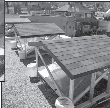
Figure 8 – Completed roof huts in place on low-slope commercial rooftop in Vancouver, BC.
