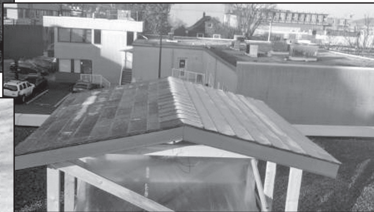
Figure 16 – Frost on exterior of shingles and impact of rising sun during the morning of January 2, 2013.
