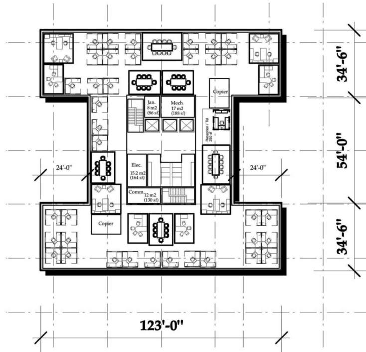
**FIGURE 3: MEDIUM H-SHAPED PLAN FORM, EAST-FACING NOTCH (MD\*\*HE-\*)
