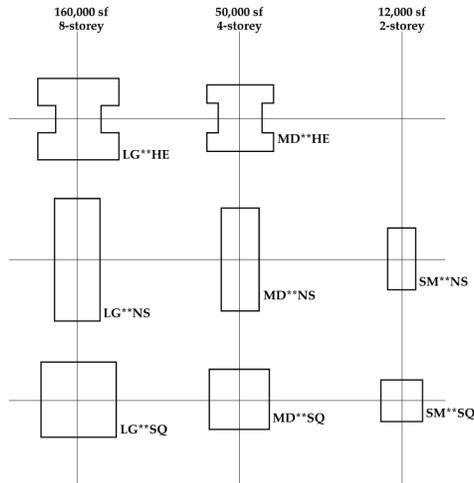
**FIGURE 2: EIGHT PLAN FORMS USED IN THIS STUDY**
