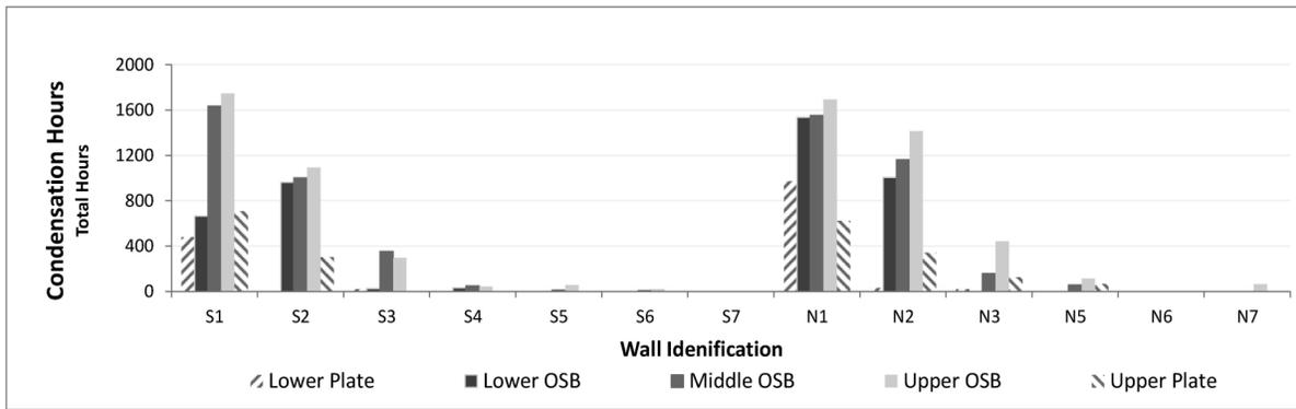
**FIGURE 6: TOTAL POTENTIAL CONDENSATION HOURS IN THE HIGH-RSI WALL ASSEMBLIES FROM NOV 20, 2012 TO JUNE 3, 2013**
