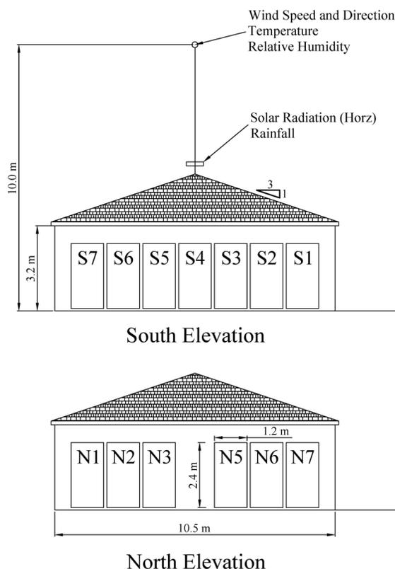
**FIGURE 1: NORTH AND SOUTH ELEVATIONS OF THE BEG HUT FACILITY ILLUSTRATING THE SIZE OF THE BUILDING AND THE POSITIONING OF THE TEST PANELS.**
