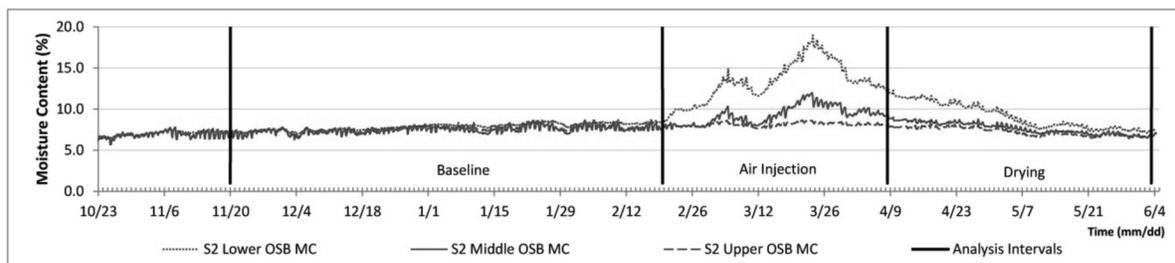
**FIGURE 5: VERTICAL OSB MC-PROFILE OF THE SOUTH I-JOIST TEST WALL S2 DURING EACH OF THE ANALYSIS PERIODS**
