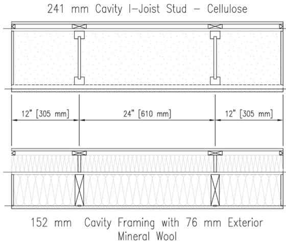
**FIGURE 2: TYPICAL PLAN DIAGRAMS OF TEST PANEL FRAMING FOR THE TYPE 2 I JOIST (TOP) AND TYPE 7 EXTERIOR INSULATED (BOTTOM)**
