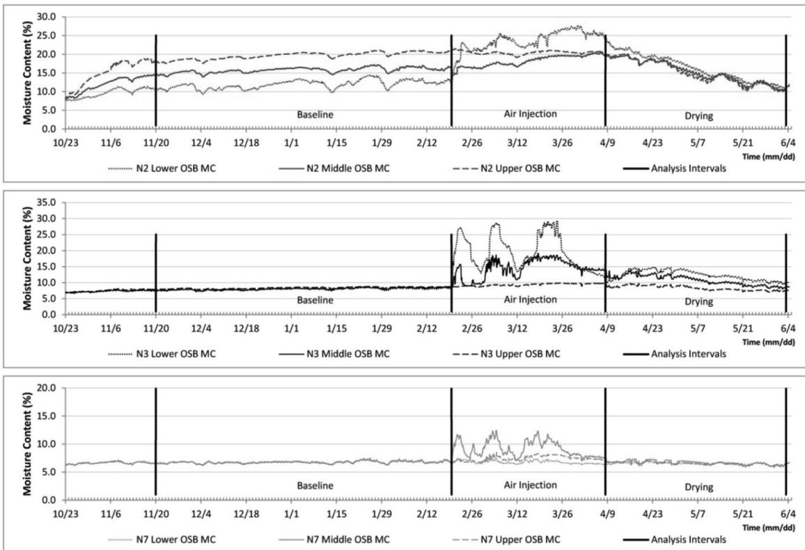
**FIGURE 4: VERTICAL OSB MC-PROFILES FOR TEST WALLS N2 (TOP), N3 (MIDDLE), AND N7 (BOTTOM)**
