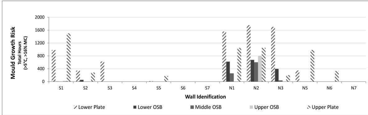
**FIGURE 7: TOTAL MOULD GROWTH HOURS (>5°C, >16% MC) FROM NOV 20, 2012 TO JUNE 3, 2013**
