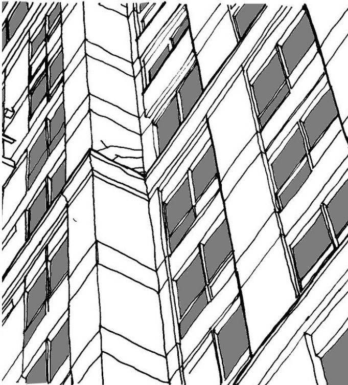
Figure 9: Example of stress fracture pattern
