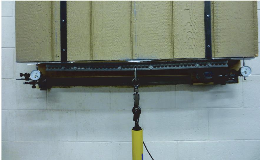
**Figure 2** Short-term deflection test setup and measurement.
