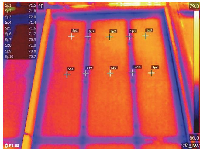
**Figure 7** Drywall surface temperatures of  $2 \times 4$  framed wall with continuous exterior R-5 fibrous insulation.
