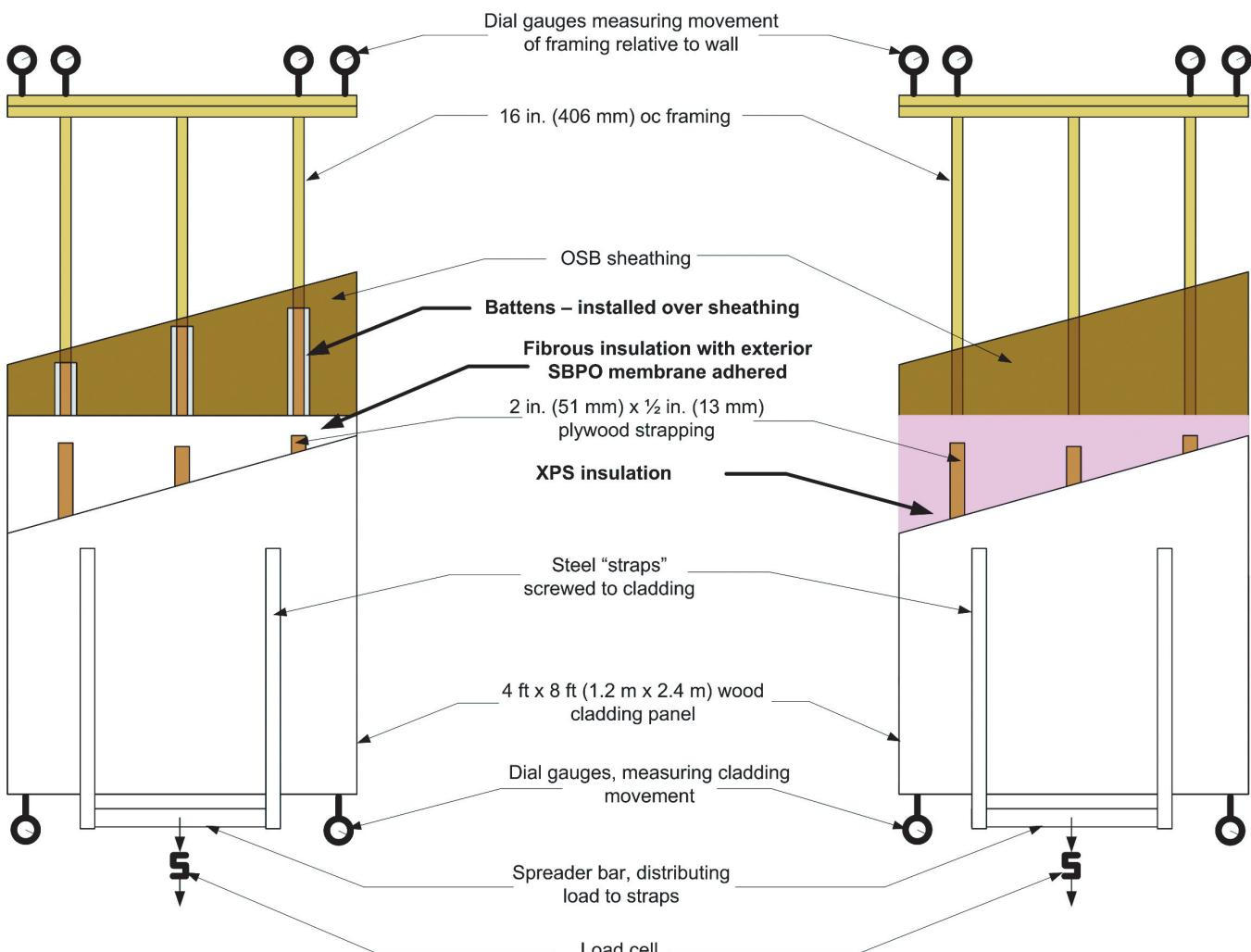
**Figure 1** Schematic construction drawing of the fibrous insulation and XPS wall assemblies for short-term deflection testing.
