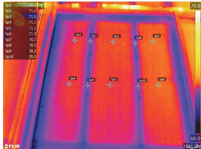
**Figure 6** Drywall surface temperatures of  $2 \times 4$  framed wall with continuous exterior R-5 XPS.
