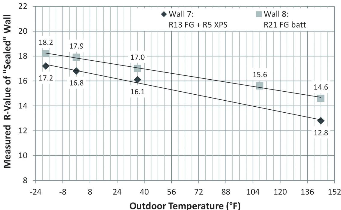
**Figure 8** Results of guarded hot-box testing of two wall assemblies (Schumacher et al. 2013).
