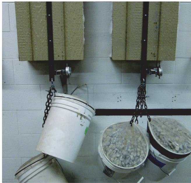
**Figure 4** Long-term deflection testing weights.
