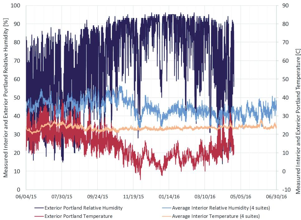
**Figure 5** Interior and exterior temperature and relative humidity (Portland).
