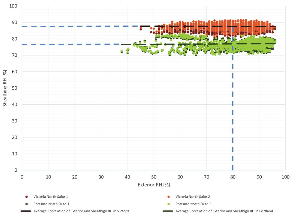
**Figure 10** Distribution of sheathing relative humidity for Victoria (orange) and Portland (green), on the north orientation.
