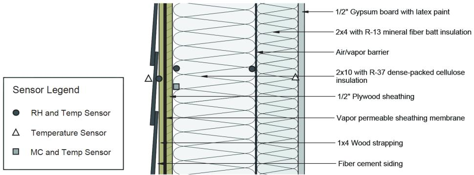
**Figure 4** Detailed assembly and typical monitoring locations (Victoria).
