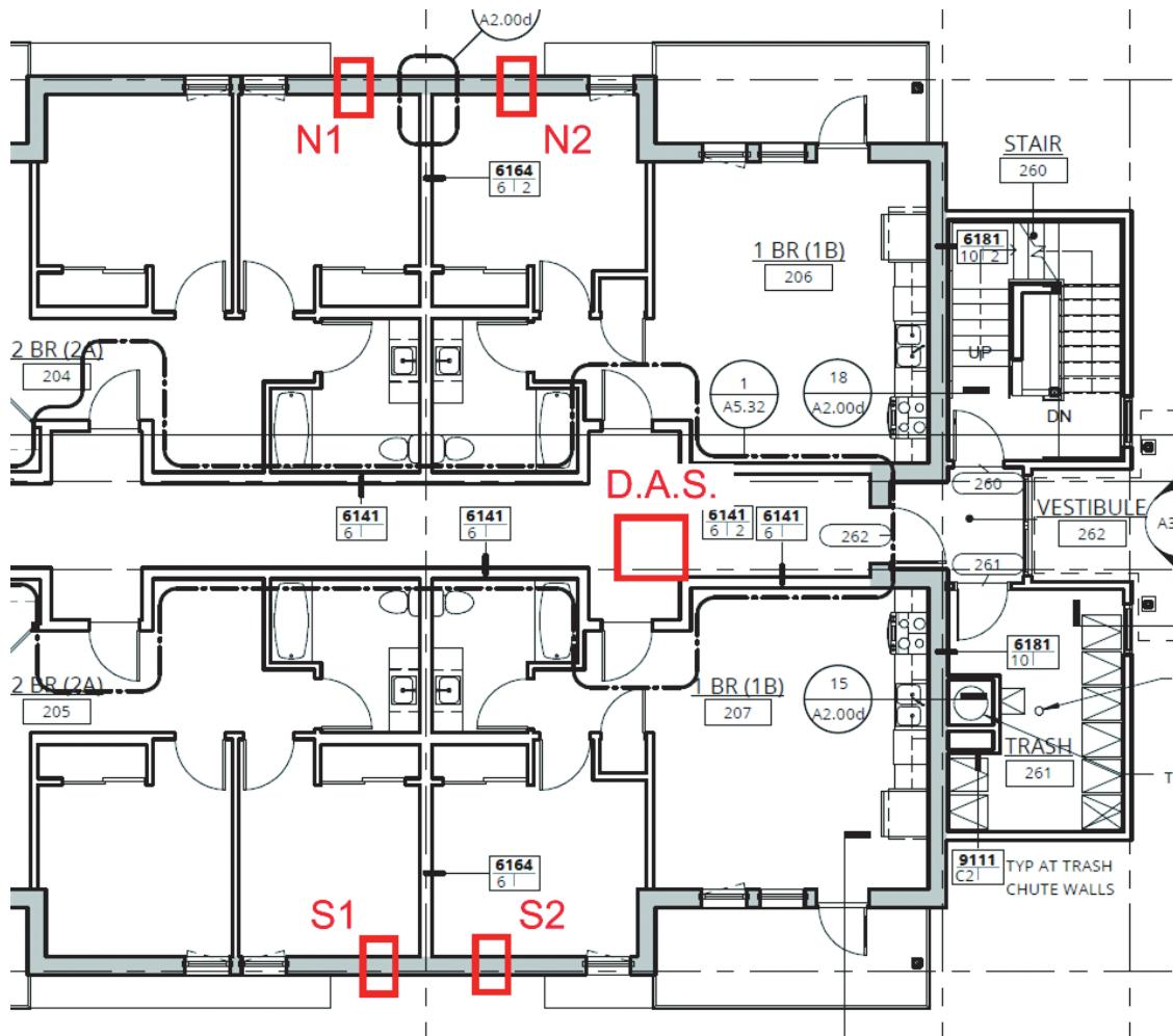
**Figure 1** Four monitoring locations and the location of the data acquisition system on the third floor (Portland).
