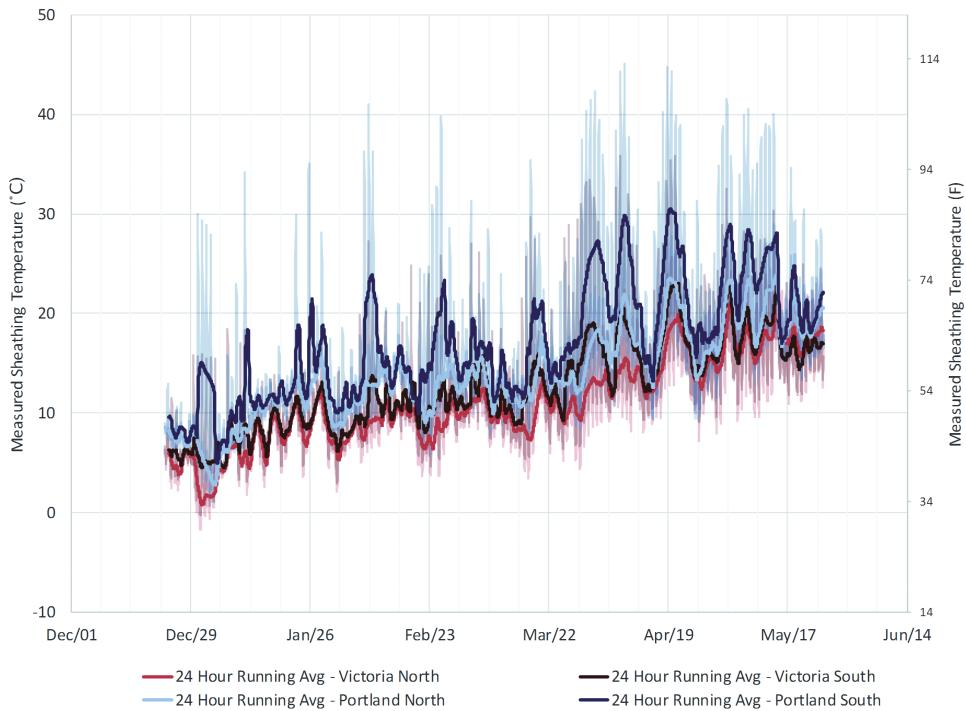
**Figure 7** Sheathing temperature and 24 h running average for Portland (blue) and Victoria (red), north and south orientations.
