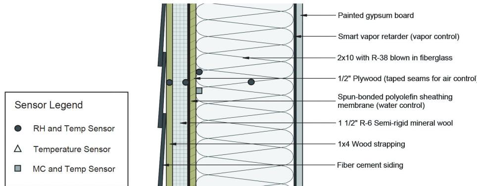
**Figure 2** Detailed assembly and typical monitoring locations (Portland).
