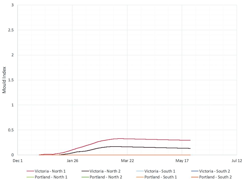
**Figure 11** Mold index results for Victoria and Portland, modeled from December 2015 to May 2016. The mold index was 0 for all four monitored locations in Portland and on the south orientation in Victoria.
