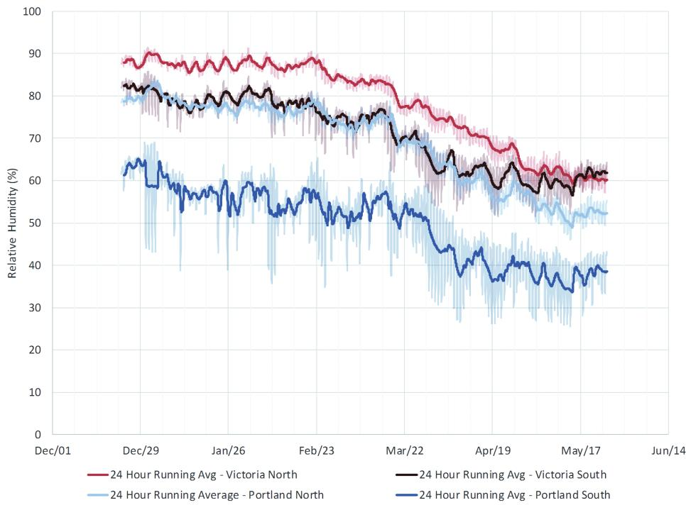
**Figure 8** Sheathing relative humidity and 24 h running average for Portland (blue) and Victoria (red), north and south orientations.
