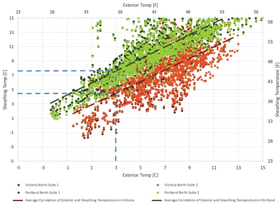
**Figure 9** Distribution of exterior temperatures and sheathing temperatures for Victoria (orange) and Portland (green), on the north orientation.
