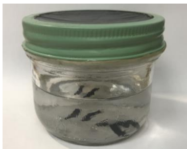
Figure 5: Example of one osmosis sample container. The membrane (black) is sealed between the powder-coated lid (green) and the glass container (clear) with epoxy. Salt water is inside the container. Samples were given code numbers, which can be seen on the bottom of this container (3.11).
