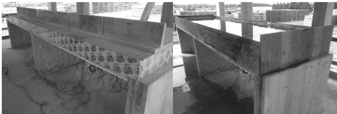
Figure 3: CLT test sample partial screed topping removal and wetting test
