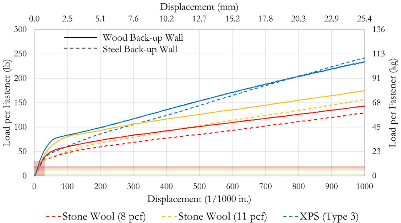
**Figure 3** Load-displacement plot comparing different insulation arrangements at 6 in. (152 mm) thickness. The plot provided in dashed line is for the second loading of each setup (steel back-up wall) and the load-displacement data from tests performed for wood frame construction (Tatara and Ricketts 2017) is provided in solid line. Note that the plot range shown in Figure 2 is highlighted by a red box.
