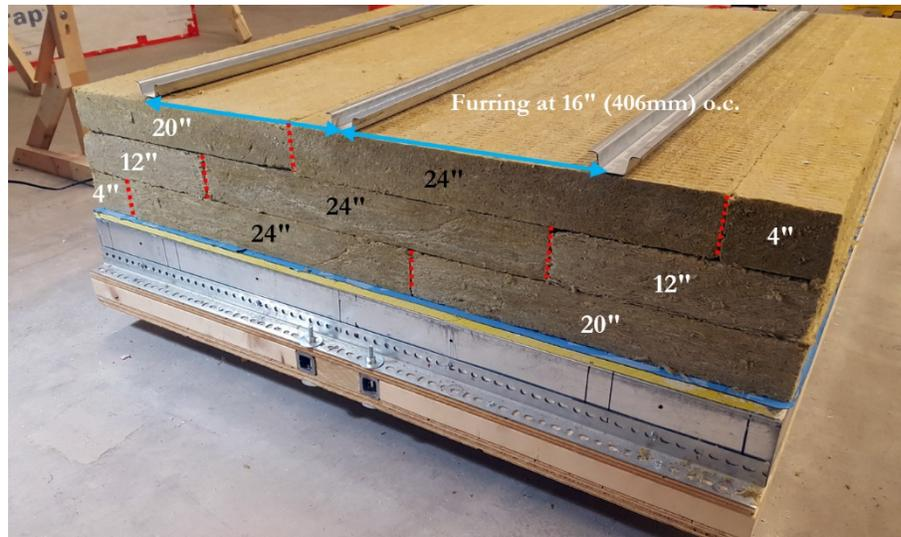
**Figure 1** An example of staggered insulation installation (9" of 11 pcf stone wool shown).
