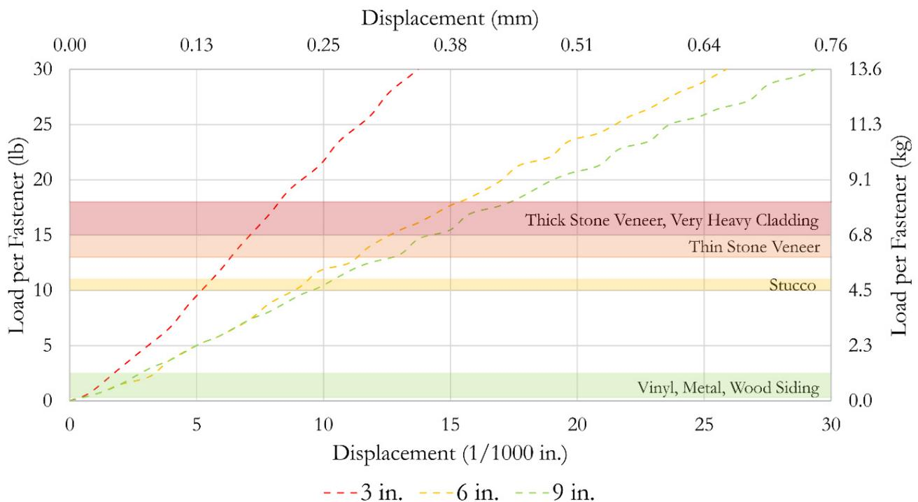
**Figure 4** Load-displacement plot comparing 11 pcf stone wool insulation at 3 in., 6 in., and 9 in. (76 mm, 152 mm, and 229 mm) thicknesses. The plot provided is for the second loading of each setup
