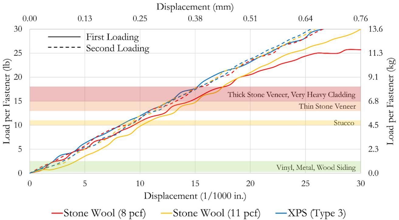
**Figure 2** Load-displacement plot comparing different insulation arrangements at 6 in. (152 mm) thickness. The plot provided is for first and second loading of each setup.
