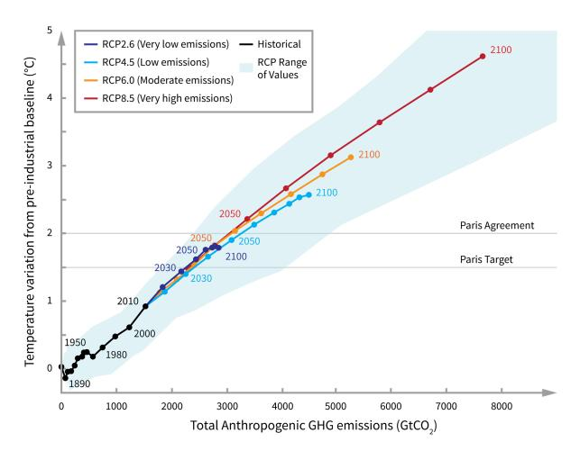
The four Representative Concentration Pathways (RCPs) described in the IPCC's Fifth Assessment Report demonstrate how an increase in cumulative CO2 emissions are associated with global temperature increases. The main difference between the RCPs is how much global warming is expected by the year 2100. The only way to return to preindustrial levels (i.e., 0°C temperature increase) is by *actively removing the excess CO*, *in our atmosphere*. Data points based on IPCC (2014), p. 55-74.
