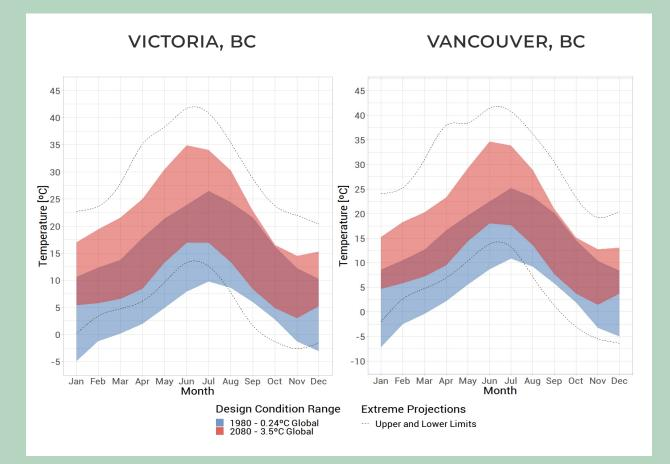
Projected local design temperatures at a global temperature of ~ $3.5^{\circ}$ C. (red) compared to the 1980 global temperature of ~ $0.24^{\circ}$ C (blue). Data from the Pacific Climate Impacts Consortium.
