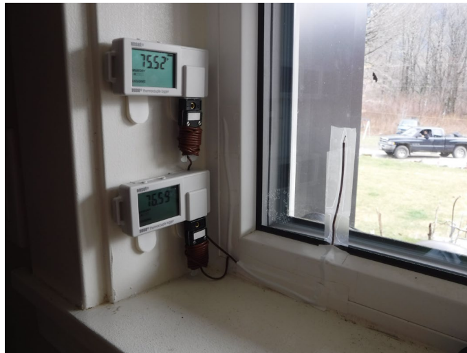
Figure 2.5 Window temperature sensors mounted to record frame and glass temperature on the fixed portion of the living room window
