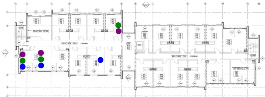
Figure 3.3 – Location of sensor installations at Building C
