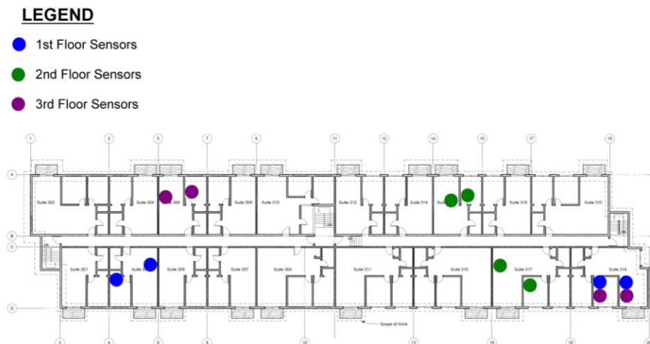
Figure 3.2 – Location of sensor installations at Building B
