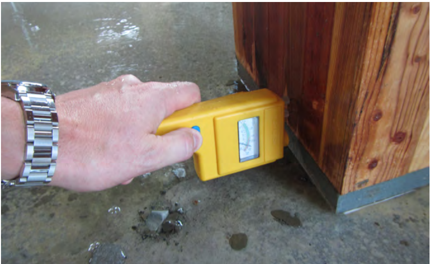
Figure 24 Moisture content reading taken at the base of a mass timber column that has been exposed to moisture; regular readings are part of the moisture exposure response plan.
