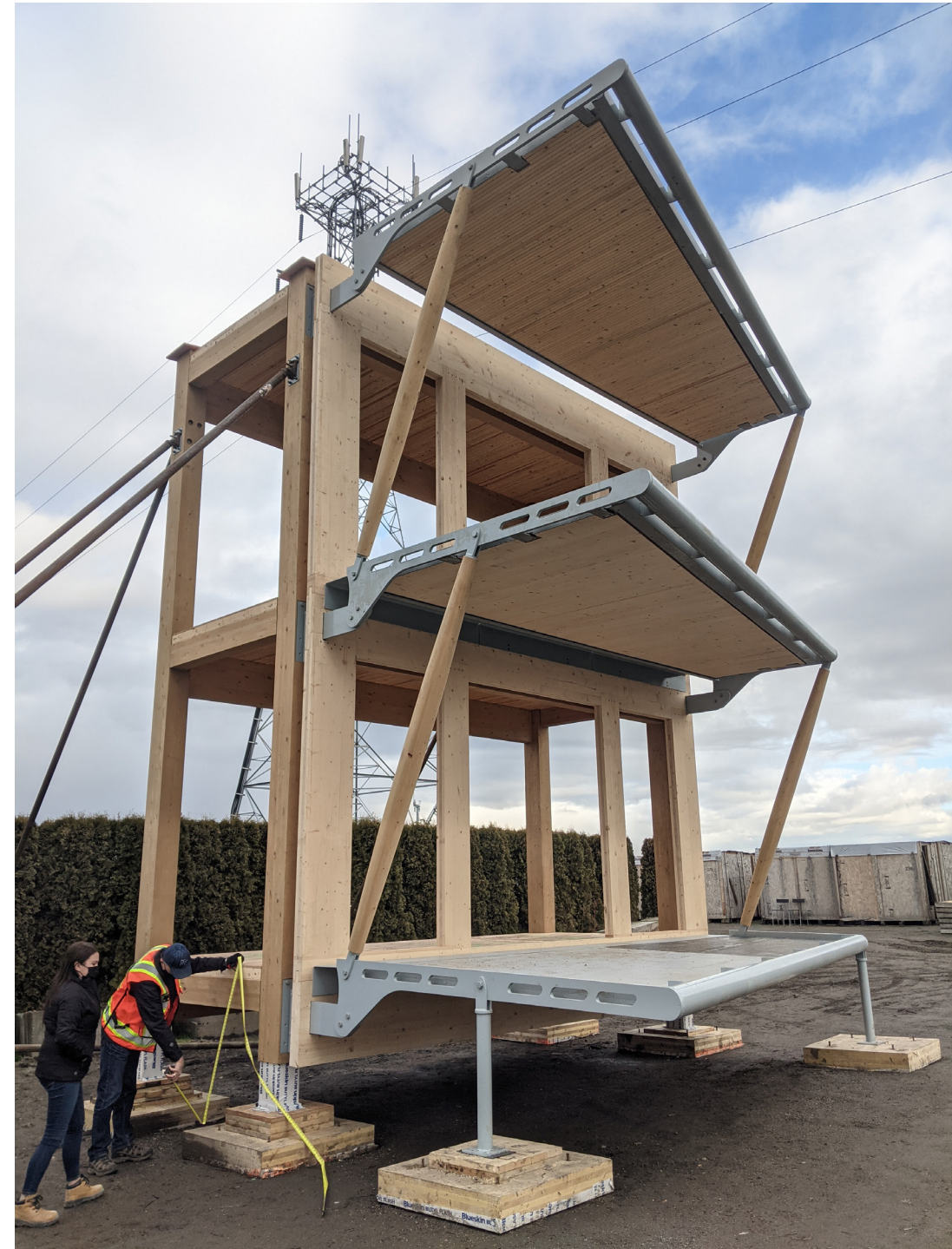
Figure 24 A two-story balcony mock-up. Visible space between the balcony elements and CLT wall panel will be filled with insulation, flashing, and cladding elements.
