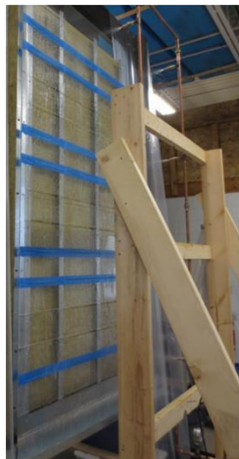
Tape joints in front of nozzles
