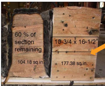
Glulam beam after 90 min fire test (APA)
