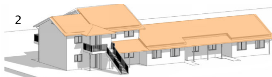
REMOVE EXISTING ROOF SHINGLES DOWN TO SHEATHING
