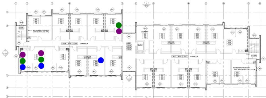
Figure 3.3 – Location of sensor installations at Building C
