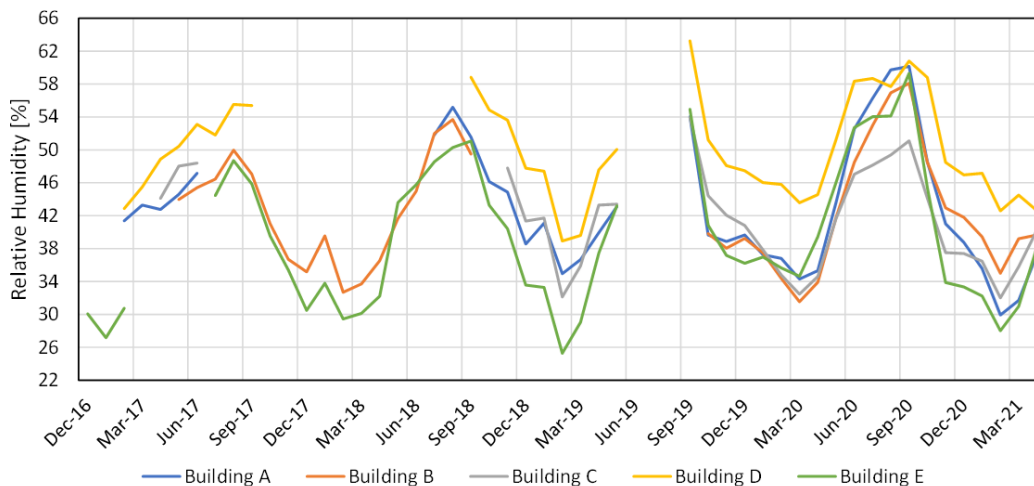
Figure 4.15 - Monthly average RH for each building. Gaps in data are either retrofit periods or missing data.
